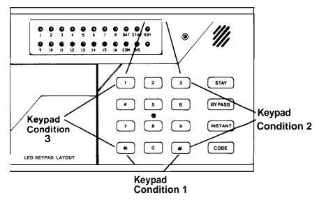
The keypad emergency conditions are programmable and can be used for conditions such as PANIC, FIRE, or MEDICAL Emergency. These conditions can be programmed by your installer to suit your needs. The keypad emergency conditions are active 24 hours a day, whether the system is armed or disarmed.
